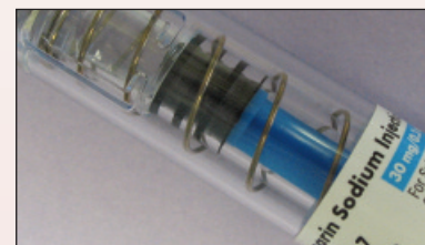
Figure 1. Syringe with spring spontaneously activated prematurely and with safety shield locked over the needle prior to use.
